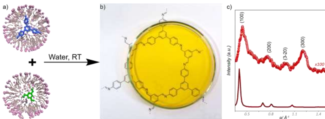
Figure 1: a) Scheme of the synthesis of TAPB-BTCA COF in micellar medium. b) Photograph showing the homogenous COF colloid in water. c) X-ray diffraction pattern of the colloidal solution containing TAPB-BTCA COF.
