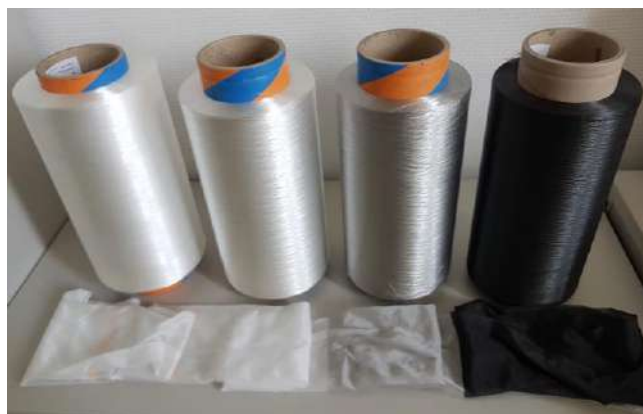
Figure 1: Melt-spun PET yarns containing various amounts of graphene.
