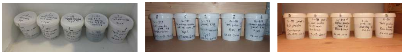
Figure 1: Samples of five different graphene oxide products stored at -18 °C, 5 °C and room temperature since May 2018, to be analyzed regularly over the coming 600 years!
