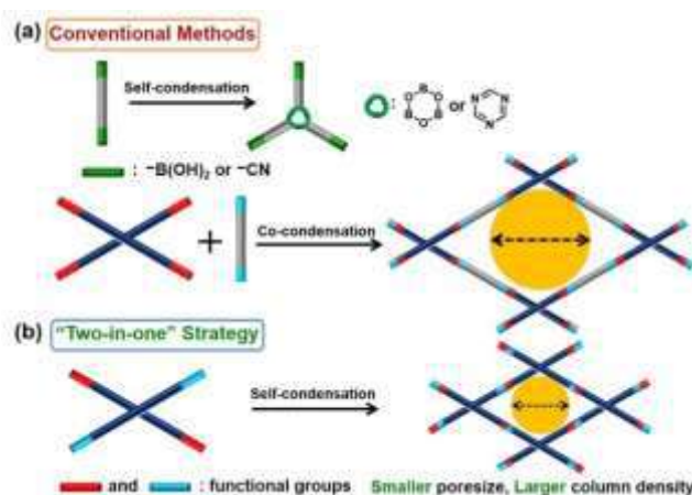
Figure 1: Schematic diagrams for 2D COFs constructed by (a) conventional self- and co-condensation methods and (b) our new two-in one strategy.
